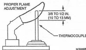
Fig. 3. Proper flame adjustment.
