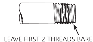
Figure 1. Pipe Compound Application
