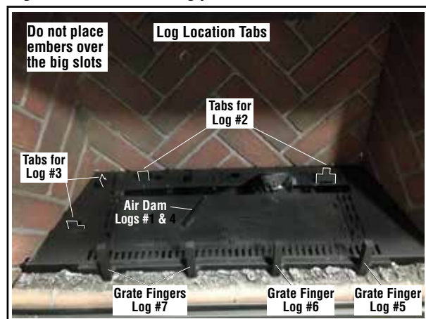
Figure 41 - Locate the log placement tabs
