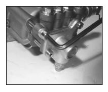
4. Next, remove the four manifold bolts (40) with a 6mm allen wrench.
