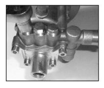
1. With a 14mm socket wrench, remove the three discharge valve plugs (27). Inspect the valve plug o-rings (23) for wear, and replace as necessary.
