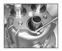
8. If the crankcase oil seals (15) are to be replaced, they can be removed by prying loose with a screwdriver. Take care not to make contact with the plunger (8) and pry out the oil seals from their housing. Seals should not be reinstalled until after step #16.
