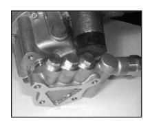
Tap the back of the manifold (35) with a rubber mallet to dislodge, and slide off the plungers. (8).
