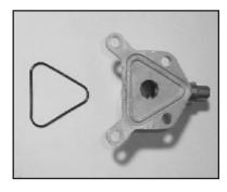
5. Remove the suction flange 6. (39) and flange o-ring (38). Inspect the o-ring for wear and replace as necessary.
