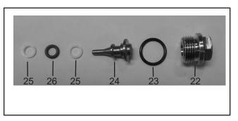
7. Remove the piston (24), o-ring (26), and backup rings (25). Remove the bypass valve seat (28). Inspect the parts for wear and replace as necessary. IMPORTANT! Make sure that the shoulder on bypass valve seat (28) is facing the discharge plug (22).
