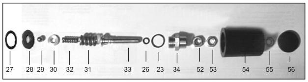
4. With a 19mm wrench, remove the adjusting screw plug (34). Unscrew the adjusting screw (33) from the adjusting screw plug (34). Inspect the o-rings (23 & 26) for wear and replace as necessary.
