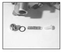
Remove the valve spring (18) and valve cone (36) from the manifold (35). Inspect the parts for wear and replace as necessary.
