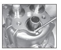
12. If the crankcase oil seals (15) are to be replaced, they can be removed by prying loose with a screwdriver. Take care not to make contact with the plunger (8) and pry out the oil seals from their housing. Seals should not be reinstalled until after step #13.
