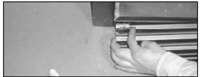
Figure 13 - Control Access Panel Removal
