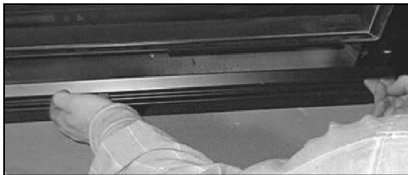
Figure 12 - Control Access Panel Removal
