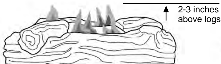
Fig. 22 - Correct Burner Flame Pattern
