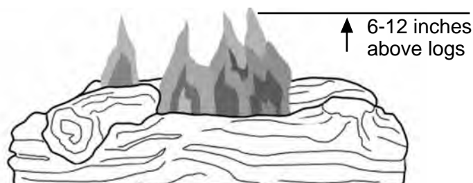
Fig. 23 - Incorrect Burner Flame Pattern
