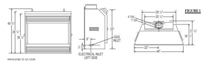
Minimum clearance to combustible construction from fireplace and vent surfaces: sides, back, bottom, and top 0 inches vent pipe 1 inch recessed depth 22 inches
