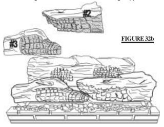
Logs (#2) and (#3) have one leg on each underside that fits into the rectangular cutouts on the burner securing plate.
