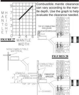
1" clearance to combustibles from the vent pipe must be maintained .
