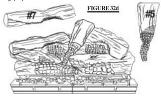
Logs (#5) and (#7) fit onto the indentations of the lower logs.
