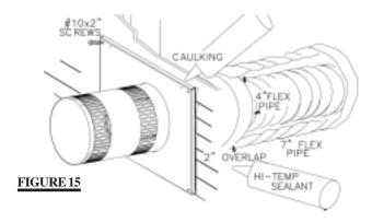
6. If more than one length of liner needs to be used to reach the fireplace, couple them together as illustrated. Seal the joints using the same procedure as described in points 2 and 3. The vent system must be supported every 3 feet, for both vertical and horizontal runs. Use Napoleon support *W010-0370* or equivalent noncombustible strapping to maintain the 1" clearance from combustibles as well as to prevent sagging.
