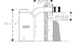
When venting, the immediate horizontal run must be kept to a minimum of 10 inches or a maximum of 3 feet.
