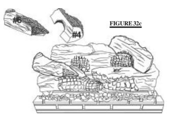
Log (#6) has a leg that fits into an indentation on the top of log (#3).
