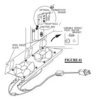
If the fireplace was not previously equipped with a fan: route a grounded 2-wire, 60hz power cable to the junction box. At this point, it must be strain relieved and insulated.
