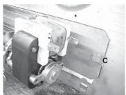
Attach and secure the variable speed switch using the nut provided. Plug the harness cord into the receptacle. The wire harness provided in this kit is a universal harness. When installed, ensure that any excess wire is contained, preventing it from making contact with moving or hot objects.
