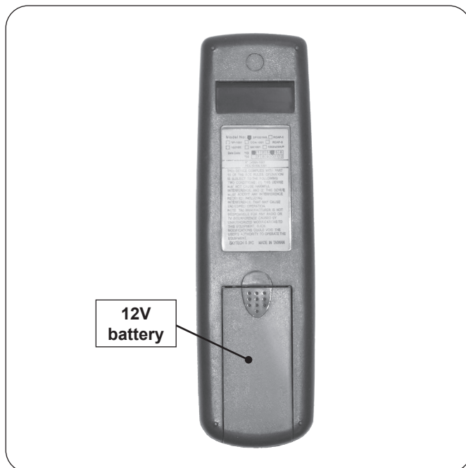
Fig. 10-1 Install transmitter battery
