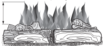
Figure 29 - Incorrect Burner Flame Pattern
