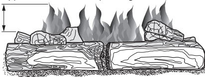
Figure 28 - Correct Burner Flame Pattern
