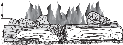
Figure 29 - Correct Burner Flame Pattern (Actual logs will vary from illustration.)
