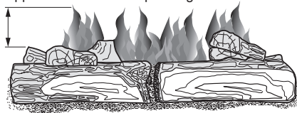
Figure 26 - Correct Burner Flame Pattern
