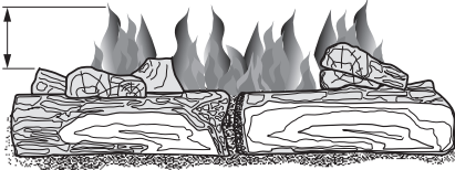
Figure 32 - Correct Burner Flame Pattern
