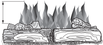
Figure 33 - Incorrect Burner Flame Pattern
