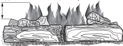
Figure 32 - Correct Burner Flame Pattern
