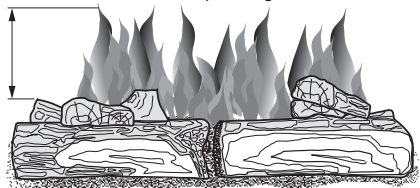
Figure 33 - Incorrect Burner Flame Pattern
