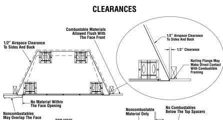
Minimum clearance to combustibles for the fireplace is as follows; sides and back - 1/2" (13mm), combustible floor - 0" (0mm), adjacent wall 6" (152mm), ceiling - 50" (1270mm).
