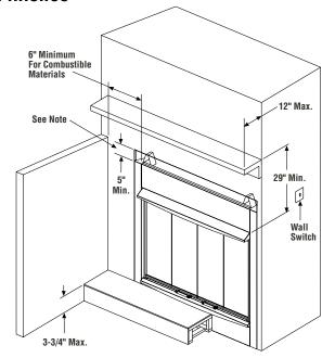
Note: The Area Above The Face To The Top Of The Spacers Must Be Non-Combustable Materials
