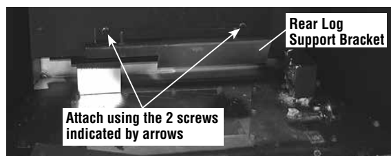
Figure 5b - Replacing Style “B” Log Bracket
