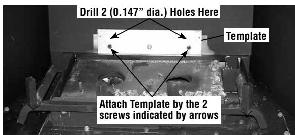
Figure 5a - Replacing Style “A” Log Bracket
