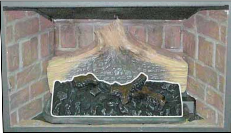
Figure 45: Place the ember bed in the center of the burner tube and pull it forward as far as it will go. Ensure it DOES NOT obstruct any part of the burner.
