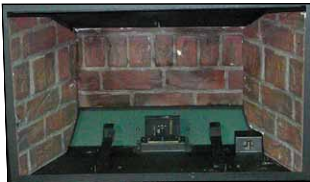
Figure 40: The side brick panels can be removed by pulling them towards the center of the firebox.
