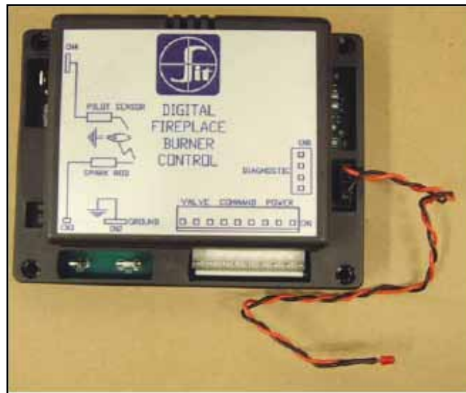
Figure 53: Proflame DFC Board with LED Indicator attached.
