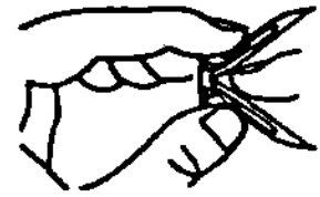
Fig. 17 - Folding the Expansion Bracket
