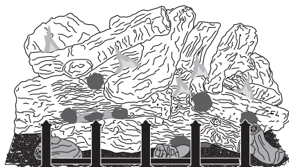
Figure 38 - Typical Flame Pattern
