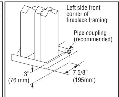
Installing the horizontal termination
