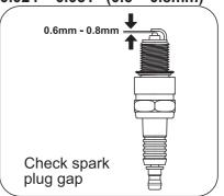
8.Carefully thread the plug into the engine **by hand.**
