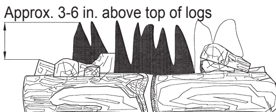
Fig. 34 - Correct Pilot Flame Pattern with Control Knob Set to High Flame (5)
