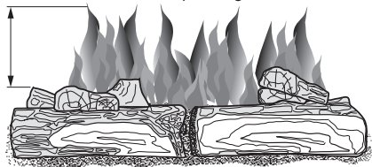
Figure 38 - Incorrect Burner Flame Pattern
