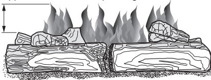
Figure 37 - Correct Burner Flame Pattern
