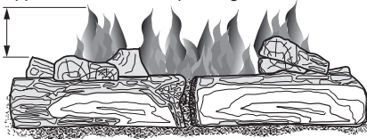
Figure 35 - Correct Burner Flame Pattern
