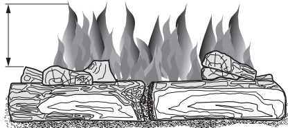
Figure 36 - Incorrect Burner Flame Pattern
