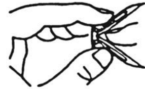
Fig. 17 - Folding the Expansion Bracket
