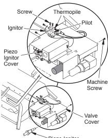
Piezo Ignitor Figure 10 - Installing Thermocouple, Pilot, and Piezo Ignitor Cover (Valve May Vary from Illustration)
