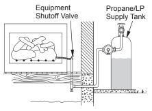
Figure 6 - Checking Gas Joints (Propane/ LP Gas Only)
