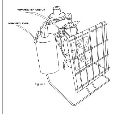
C. Turn the heater's "ON-OFF" lever to "ON".
