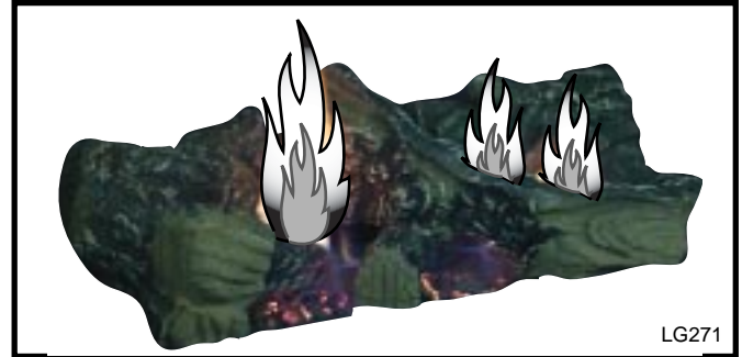
Fig. 43 Correct burner flame appearance for 33BDVT.
