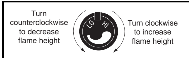
Fig. 40 Flame adjustment knob for Honeywell valve.
