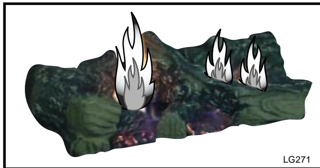
Fig. 45 Correct burner flame appearance for 33BDVR.
