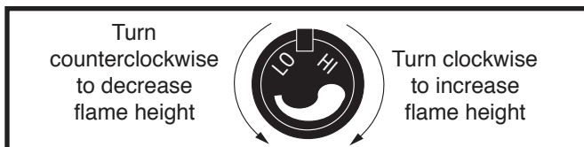
Fig. 46 Flame adjustment knob for Honeywell valve.
