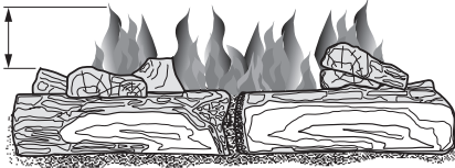
Figure 32 - Correct Burner Flame Pattern
