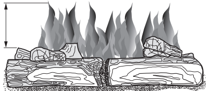
Figure 33 - Incorrect Burner Flame Pattern
