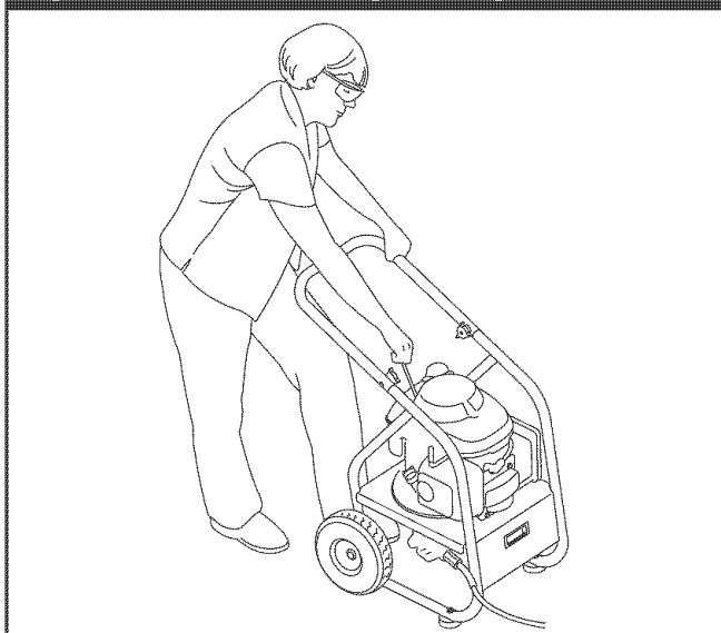
Figure 14 — Recommended Engine Starting Posture
