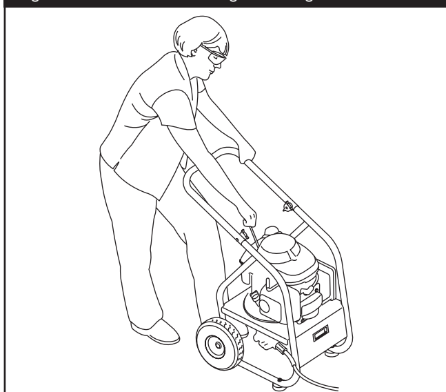
Figure 14 — Recommended Engine Starting Posture
