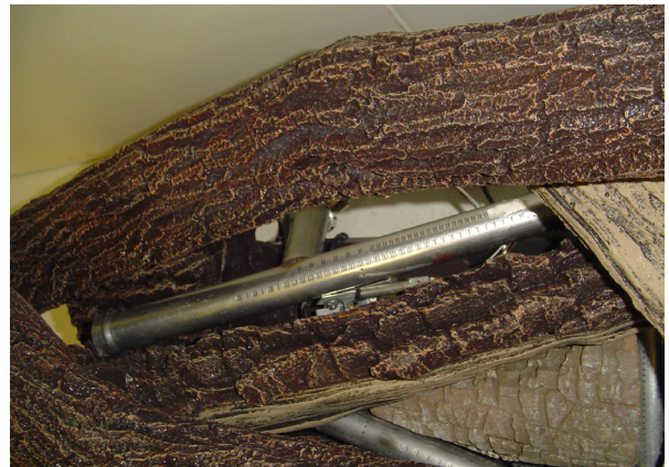
Figure 26A - Installing Back Top Log, Top View
