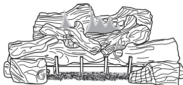
Figure 35 - Correct Front Burner Flame Pattern
