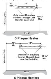
Figure 8 - Mounting bracket Clearances
