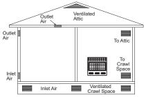
Figure 3 - Ventilation Air from Outdoors
