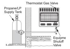
Figure 18 - Checking Gas Joints for Propane/LP Gas (actual heater may vary from illustration)
