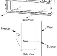
Figure 12 - Installing Bottom Mounting
