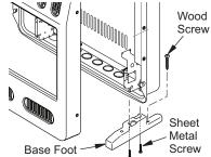
Figure 13 - Installing Base Feet (actual heater may vary from illustration)
