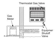
Figure 17 - Checking Gas Joints for Natural Gas (actual heater may vary from illustration)
