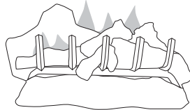
Figure 45 - Correct Burner Flame Pattern
