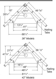
Figure 5 - Framing Clearances for Corner Installation
