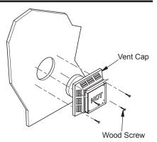
Figure 10 - Installing Horizontal Vent Cap (Noncombustible Exterior)
