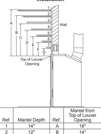
Figure 6 - Clearances for Combustible Mantels
