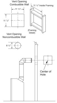
Figure 9 - Vent Opening Requirements
