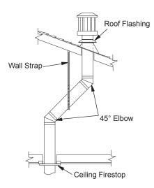
Figure 19 - Offset with Wall Strap and 45° Elbows
