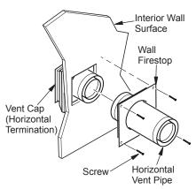
Figure 12 - Connecting Vent Cap with Horizontal Vent Pipe
