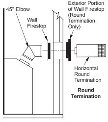
\* If installing this fireplace at altitudes of 4000 feet and above, it is recommended that an additional vertical height of 6" be added to the vent system.
