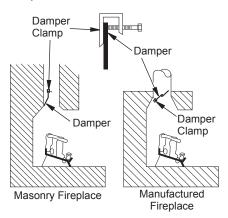
Figure 3 - Attaching Damper Clamp
