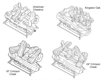
Figure 10 - Placement of Top Logs
