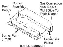
Figure 6 - Installing Burner
