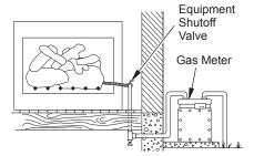
Figure 5 - Checking Gas Joints
