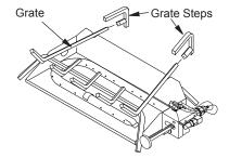
Figure 8 - Installing Grate (Pan Material Not Shown)
