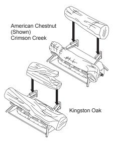
Figure 9 - Installing Front and Back Logs (Number and style may vary)
