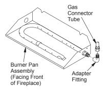
Figure 7 - Connecting Gas to Appliance
