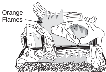
Figure 24 - Incorrect Burner Flame Pattern
