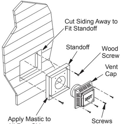
**Figure 11 - Installing Siding Standoff (Combustible Exterior Wall)**
