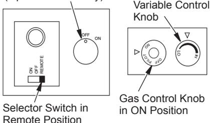
Figure 45 - Setting the Selector Switch, Gas Control Knob and Variable Control Knob for Remote Operation
