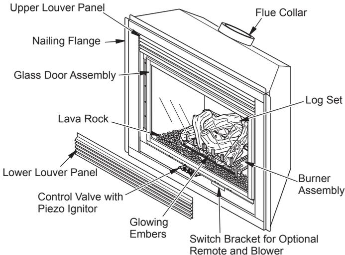
**Figure 1 - Direct-Vent Fireplace with Millivolt Ignition**
