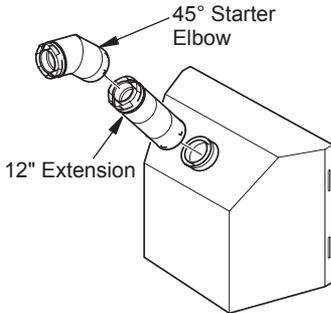
**Figure 25 - Recommended 12" Extension for High Altitude Installation**
