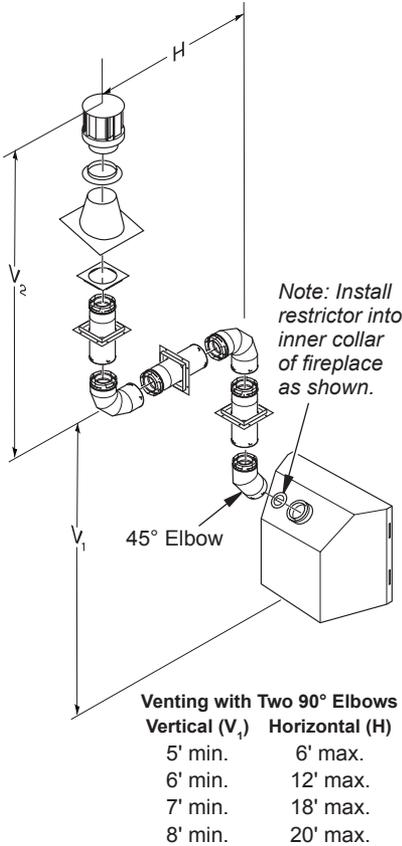
Note: Vertical ( $V_1$ ) + Vertical ( $V_2$ ) = 40' max.
