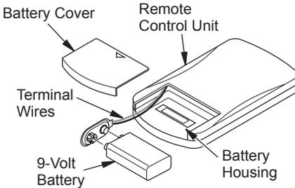
Figure 40 - Installing Battery in Hand-Held Remote Control Unit
