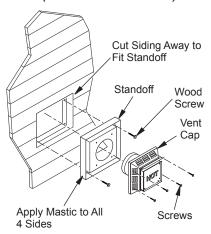
Figure 11 - Installing Siding Standoff (Combustible Exterior Wall)
