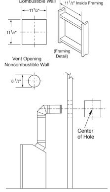
Figure 9 - Vent Opening Requirements
