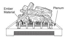
Figure 39 - Placing Ember Material on Burner
