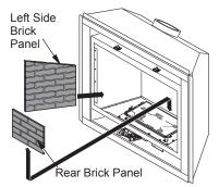
Figure 40 - Installing Rear Brick Panel
