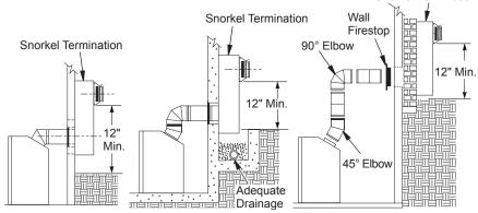
Figure 16 - Snorkel Termination Configurations for Below Ground Installation
