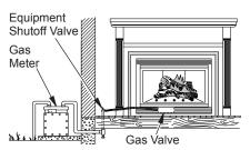
Figure 35 - Checking Gas Joints for Natural Gas Fireplace
