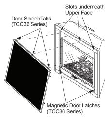
Figure 37 - Removing/Replacing Screen Door Assembly (TCC36 Series)
