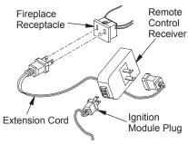
Figure 41 - Installing the WRC Remote Receiver
