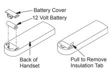
Figure 42 - Installing Battery into Back of Handset
