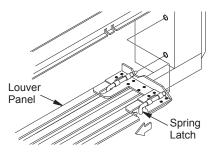
Figure 36 - Removing Louver Panel
