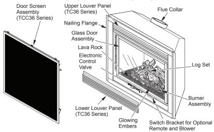
Figure 1 - Direct-Vent Fireplace with Electrionic Ignition
