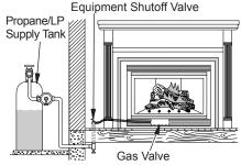
Figure 34 - Checking Gas Joints for Propane/LP Gas Fireplace
