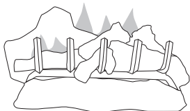
Figure 12 - Correct Burner Flame Pattern
