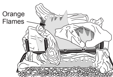
Figure 24 - Incorrect Burner Flame Pattern
