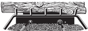
Ignitor Button Control Knob Figure 32 - Control Knob and Ignitor Button Location
