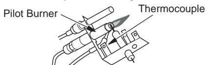
Figure 31 - Correct Pilot Flame Pattern (Your pilot may vary from pilot shown)
