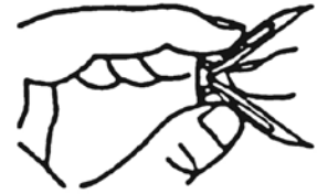
Fig. 17 - Folding the Expansion Bracket
